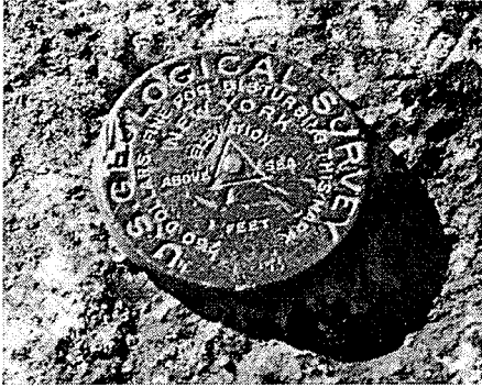
One of three U. S. Geological Survey bench marks on the summit of Arab Mountain.
